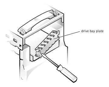
Remove the extra rails from the front of the computer frame (see the illustration below).
